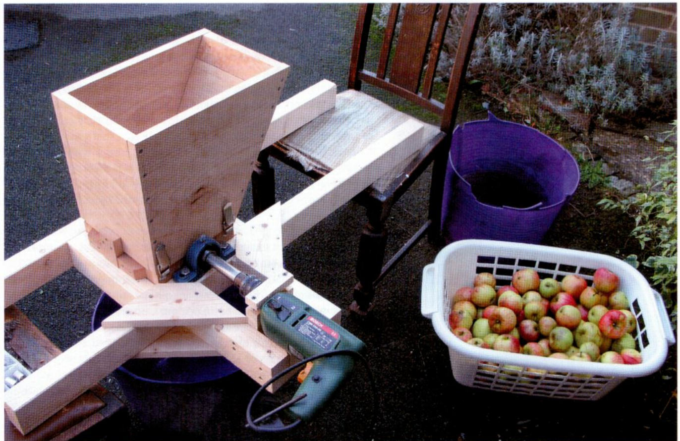
Below: DIY apple scratter (chopper/masher) powered by an electric drill.
