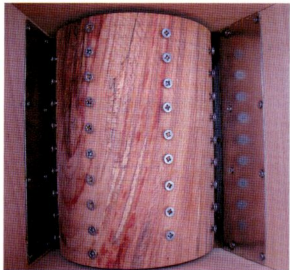
Bottom: Hopper (upside down) showing stainless steel sheets.
